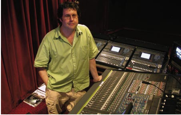
Michael Waters behind the PM5D-RH used for the world premiere of Dirty Dancing . Behind him are three Yamaha DM1000s taking care of the band submixes.
