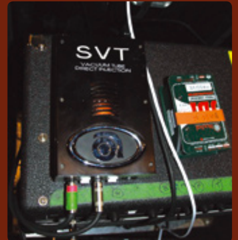
With two Ampeg SVT bass heads, nothing would do but an Ampeg SVT Tube DI, the Radial is a spare. All DI boxes are not equal.
