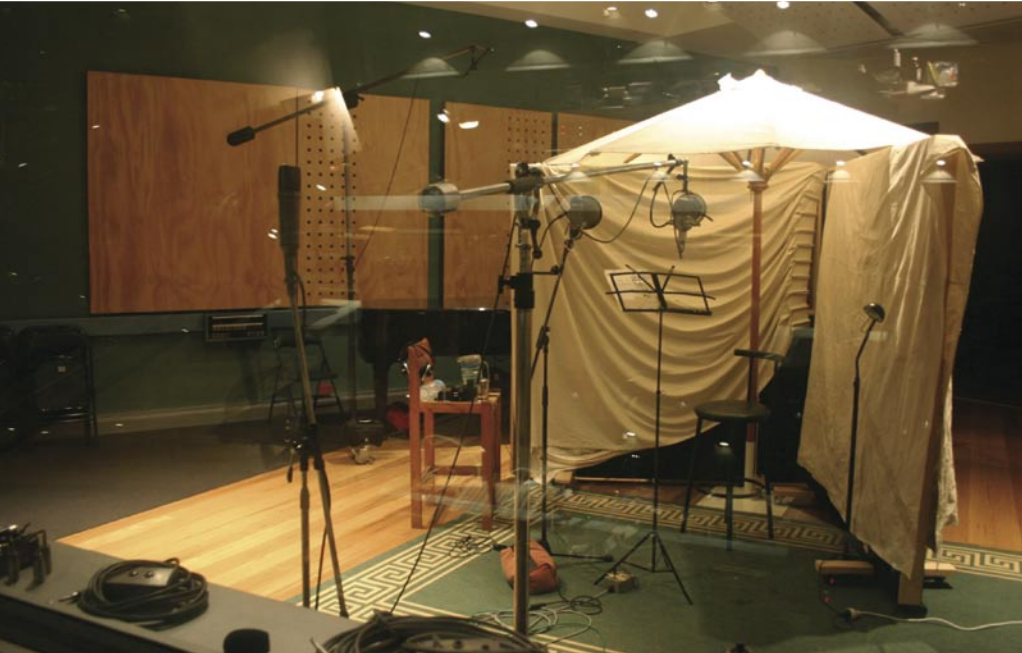
Camping out in Camperdown: The main recording room at Electric Avenue in Camperdown, Sydney hosted many of the main tracking and overdub sessions. Vocals were often recorded under a beach umbrella to minimise the ambience around the vocal mic. The vocal mics under the 'bigtop' (pictured above) include a Neumann M49 & U87 and an AEA R84 ribbon.
