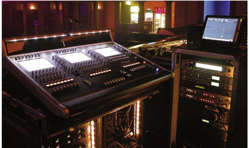
The FOH position, dominated by the Digico D1. You'll notice the Clair IO in the rack. It was used purely for its EQ; the PA system control was all done from within the Digico D1.
