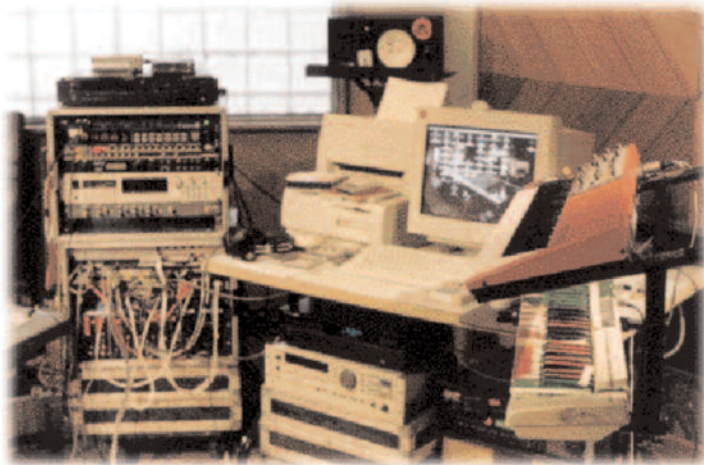
Rob’s preproduction set-up. Among others you’ll notice an Akai S3000, Novation DrumStation, Roland JV1080, an Alesis D4, a Panasonic SV3800 DAT recorder and the distinctive Nord Lead in the foreground. Note the keyboard under the Nord mashed beyond all recognition, sporting a Rob Taylor ‘retrofit’.
