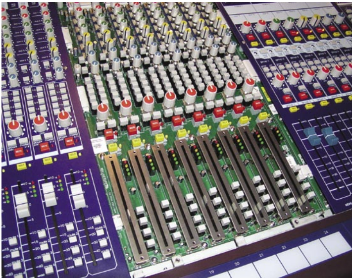
The Verona's faceplates can be removed easily to facilitate cleaning.
